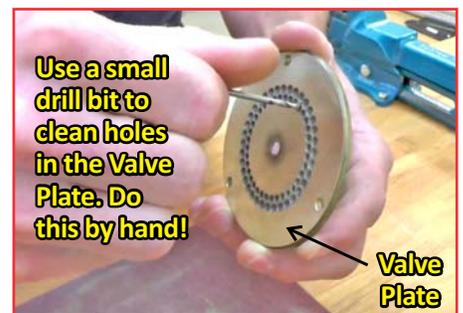
Use a small drill bit to clean holes in the Valve Plate. Do this by hand!
