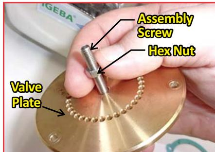
To take the Air Intake Valve apart, remove the hex nut and assembly screw.
