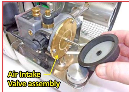
Removing the Knurled Nut and Silencer Cap reveals the Air Intake Valve assembly.
